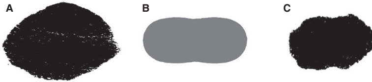
Figure 5 IRE versus H-FIRE ablations in potato tuber. A qualitative comparison between an IRE ablation and an H-FIRE ablation created using a single bipolar probe. (A) IRE was induced with 80 pulses energized for 100 \mu s at 1000 V. (B) Laplace solution for the electric field distribution at an arbitrary electric field magnitude, assuming static electrical conductivity. (C) H-FIRE was induced with 140 bursts, using a burst scheme of 2-5-2 \mu s at 1300 V. Typical H-FIRE protocols require higher voltages and more bursts to produce lesion volumes comparable to IRE.
