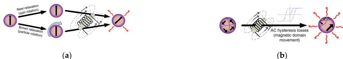
Figure 3. Schematical representation of heat release mechanisms under AMF effect in (a) single-domain MNPs and (b) multi-domain MNPs.
